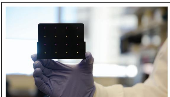
**Fig. 1.** A black cartridge containing a paper-based diagnostic for detecting the Zika virus is held up by a researcher at Harvard's Wyss Institute.
